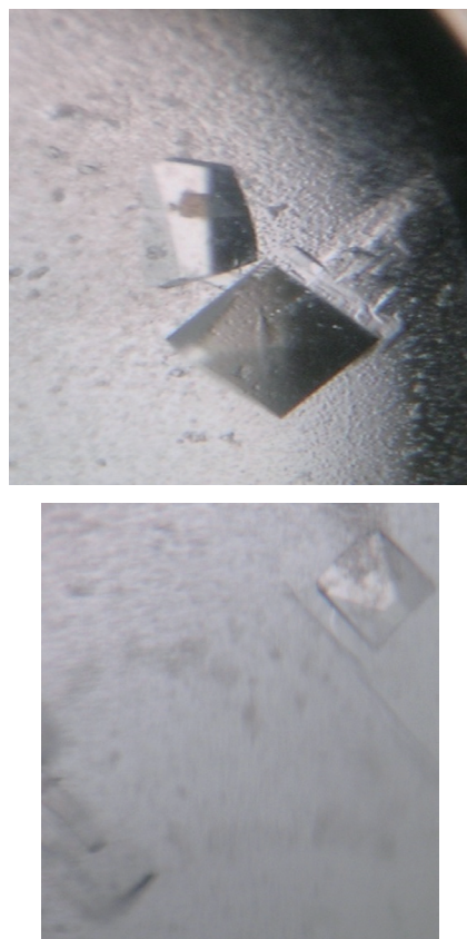
FIGURE 2 | Crystals of Csm5. The crystals were obtained in two week using a reservoir solution containing 20 % PEG 8000 (w/v), 100 mM CHES/sodium hydroxide pH 9.5 at 291 K.
