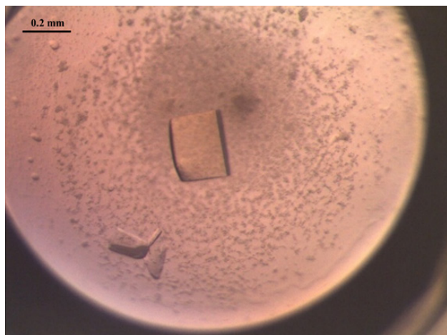
FIGURE 2 | Monoclinic crystals of the T. maritima Rex. The crystals with the best quality were obtained in 20% (w/v) PEG 3350 and 200 mM potassium chloride using the sitting-drop vapour-diffusion method at 296 K. Their approximate dimensions are 0.2 mm x 0.16 mm x 0.15 mm.
